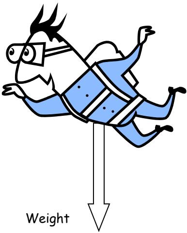
When the parachutist has just jumped from the plane, he is not yet moving so there is no drag, but only his weight. Hence he has a resultant force (downwards!!) and so he starts to accelerate downwards.
