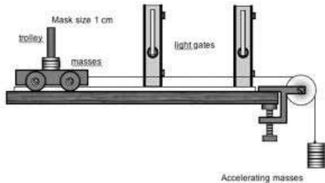
The masses on the end of the string apply a force to the trolley, causing it to accelerate. The light gates measure the velocity of the trolley as it passes through them. If we also record the time taken for the trolley to pass between the light gates, then we have measurements of initial velocity (u), final velocity (v) and time (t). We can therefore find acceleration using the equation:
