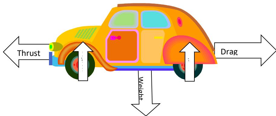
The car is moving at constant velocity. This means that it is not accelerating and so the thrust force must be equal to the drag so that the resultant force on the car is zero.
