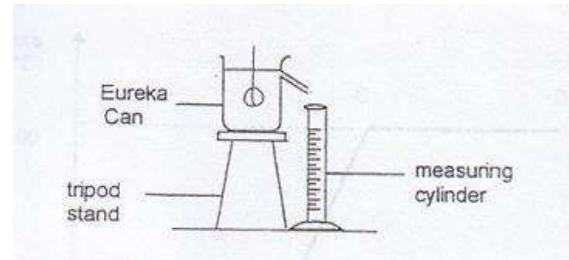
This piece of apparatus is named after Archimedes' famous exclamation when he first realised how to measure the volume of an irregular solid.
