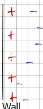
The negative charges (electrons) at the surface of the wall are repelled by the negatively charged balloon (like charges repel).
