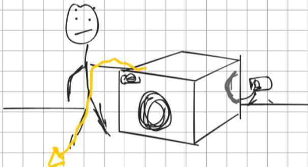
If the live wire comes into contact with the metal casing of an appliance, the casing also becomes **LIVE**.
