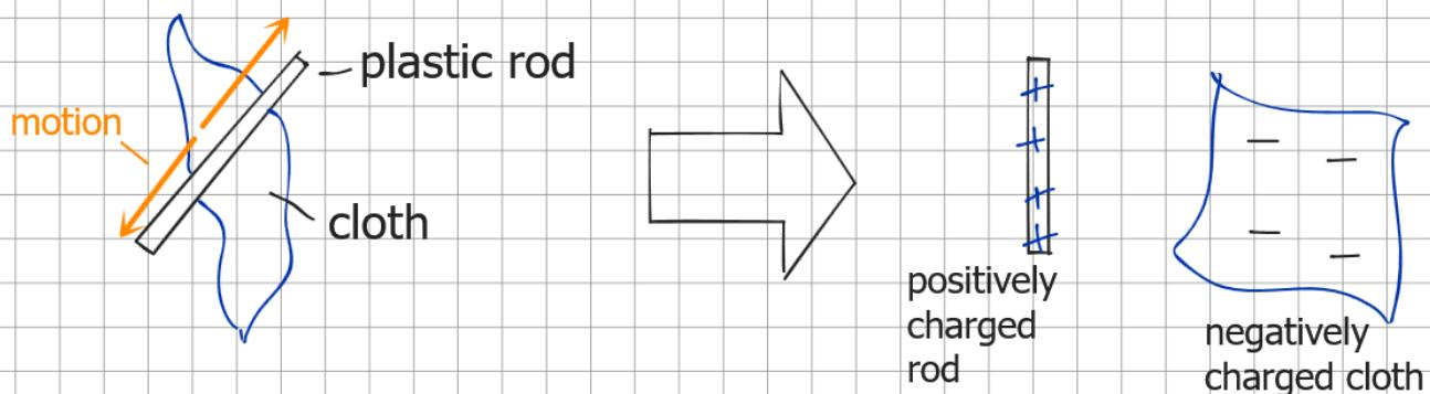
In this example ELECTRONS were transferred FROM THE ROD and TO THE CLOTH.
