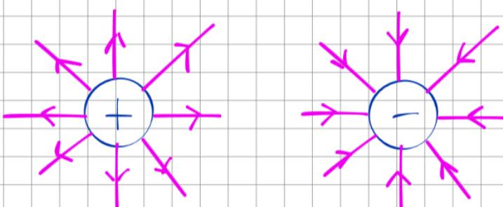
The field is stronger closer to the charged object, which is shown in the diagram as the field lines get closer together.
