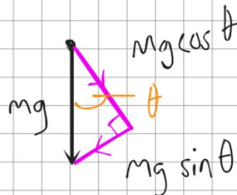
The restoring force acts tangentially to the arc that the pendulum moves through.
