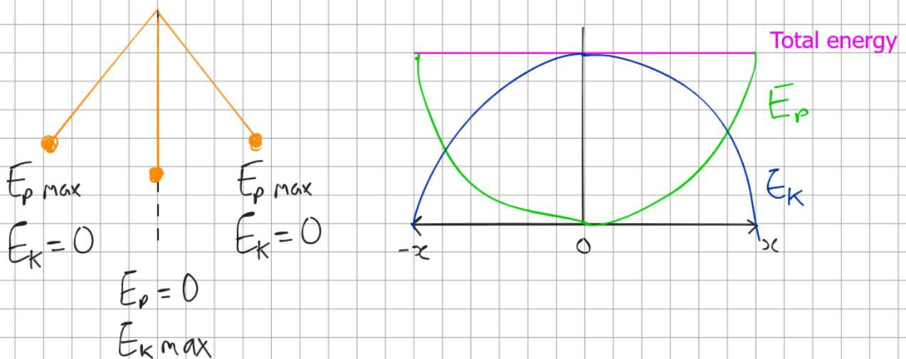
The work done to displace the pendulum to its amplitude tells us the total energy stored in the system.
