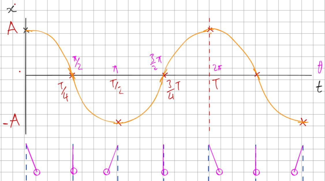
The graph above is a displacement time graph for an object undergoing SHM.
