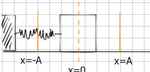
Mass oscillating horizontally on a frictionless plane.
