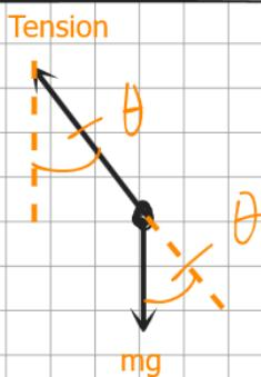
Resolving the weight into two components; parallel to string and normal to string:
