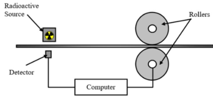
The computer monitors the count rate and adjusts the separation of the rollers appropriately.
