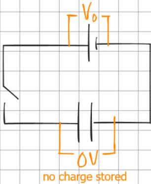
After the switch is closed charge flows and builds up on the plates of the capacitor.
