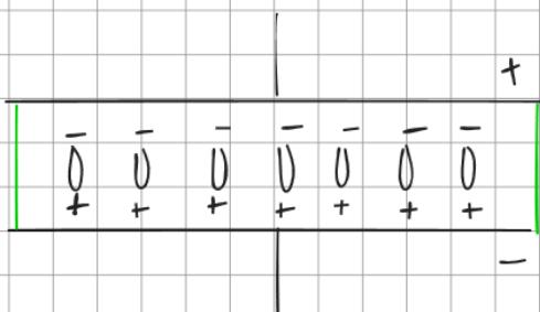
When the capacitor is charged the polar molecules align with the electric field between the plates.
