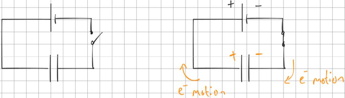
When the switch is closed electrons are pulled from one of the plates of the capacitor and forced on to the other plate. The side of the capacitor that loses electrons becomes positive, and the side that gains them becomes negative.
