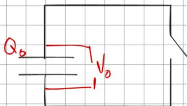
When this switch is closed the rate at which charge leaves the plates is at a maximum.
