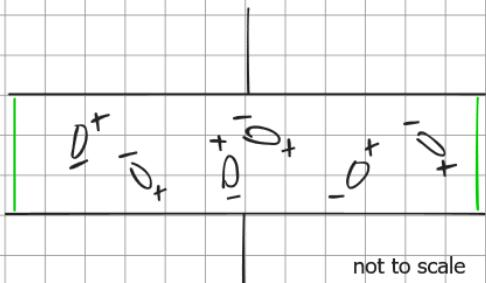
When the capacitor is not charged the molecules of the dielectric are randomly orientated.
