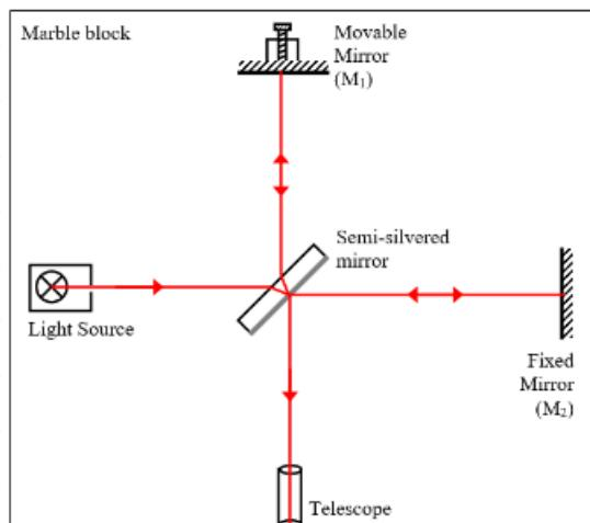
The interferometer light is directed towards a semi-silvered mirror.
