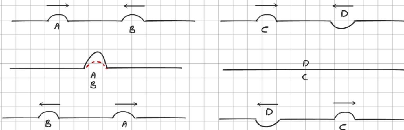
When the crests of two waves of EQUAL WAVELENGTH meet, the waves are said to be IN PHASE. If the waves have the same amplitude, the waves combine CONSTRUCTIVELY leading to a single crest with twice the amplitude.
