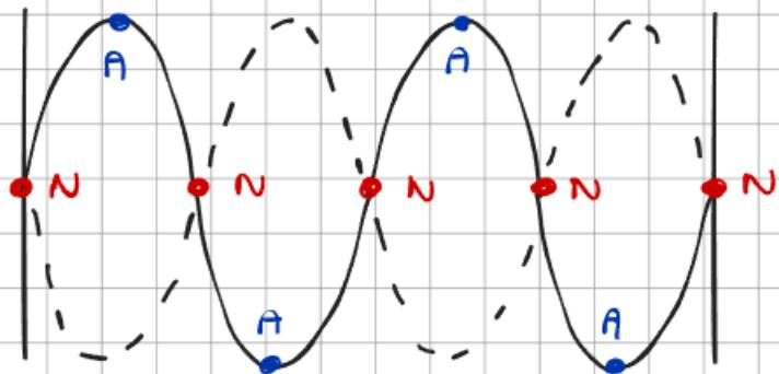
Each point on a stationary wave alternates between the solid line and the dashed line, so neighbouring points have different amplitudes.
