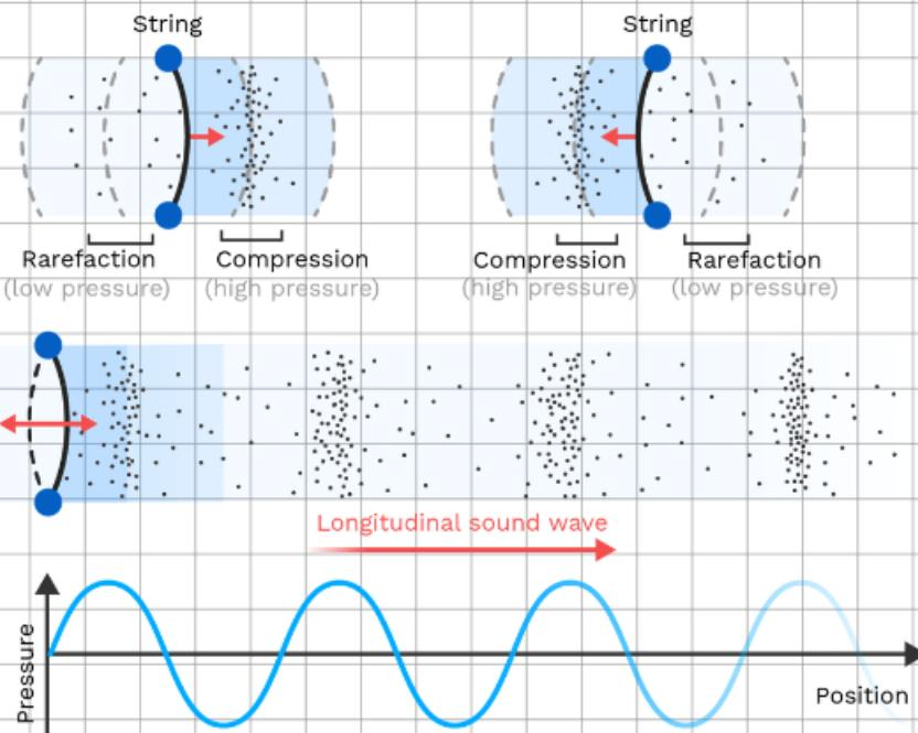
Displacement of the particles or field(s) is **PARALLEL** to the axis of propagation (direction of energy transfer).
