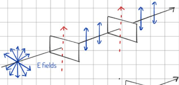
If the plane of polarisation of the second filter is also vertical ( $\alpha = 0^\circ, 180^\circ$ ) then the transmitted light will be maximum.
