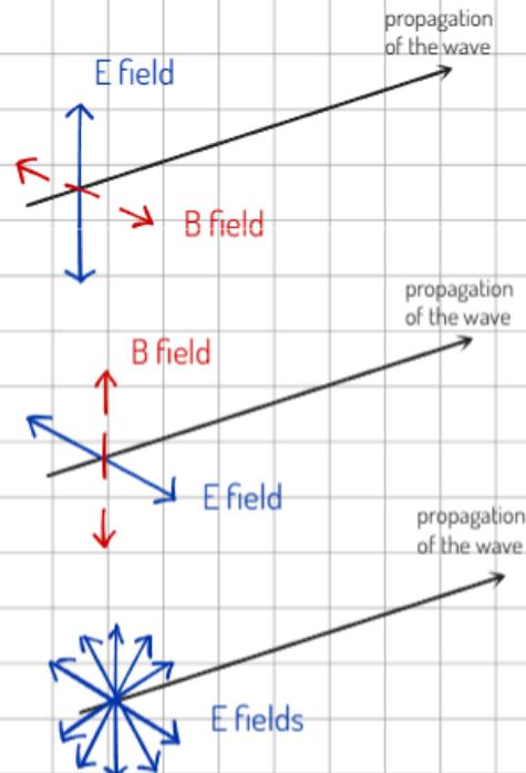
Arbitrary directions of polarisation can be RESOLVED into horizontal and vertical polarisations.
