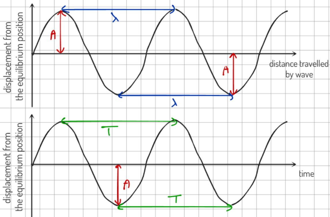
Amplitude - maximum displacement from the equilibrium position within a cycle
