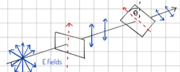
At intermediate angles some of the light is transmitted, because the vertically polarised light can be resolved so that it has some polarisation component in the direction of the transmission axis of the second filter.
