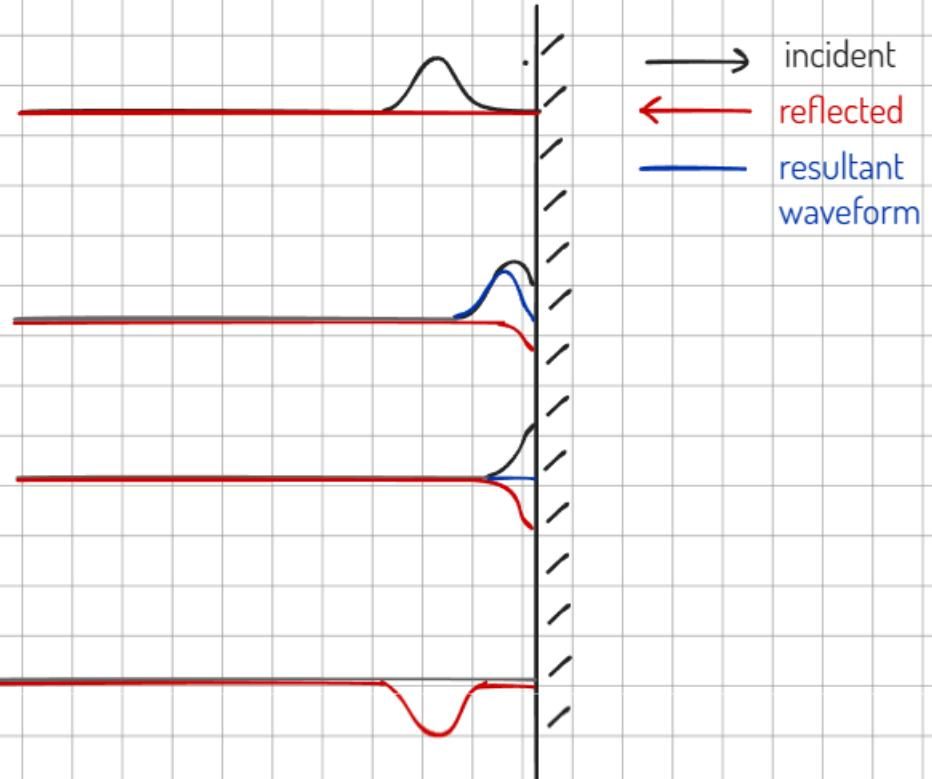
This leads to the reflected pulse being in anti-phase with the incident pulse.
