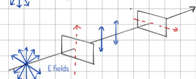
If the plane of polarisation of the second filter is also vertical ( $\alpha = 90^\circ, 270^\circ$ ) then the transmitted light will fall to zero.
