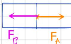
Object A exerts a force on Object B, therefore Object B exerts a force on Object A that has the same magnitude but is in the opposite direction. (According to N3L)
