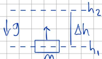
$$\begin{aligned} \Delta E_P &= mgh_2 - mgh_1 \\ &= mg(h_2 - h_1) \\ \Delta E_P &= mg\Delta h \end{aligned}$$
